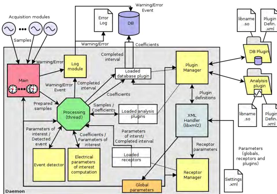
Fig. 3. Block diagram of the processing subsystem.
